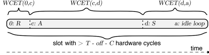
Figure 21: Worst Case Execution Time (WCET) Constraint
