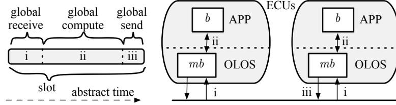
Figure 22: COA: Slot Partitioning and Data-Flow
