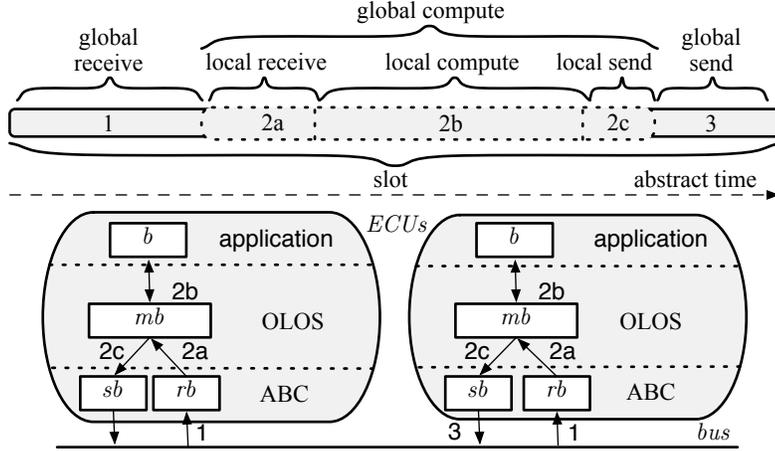
Figure 20: DOLOS: Slot Partitioning and Data-Flow
